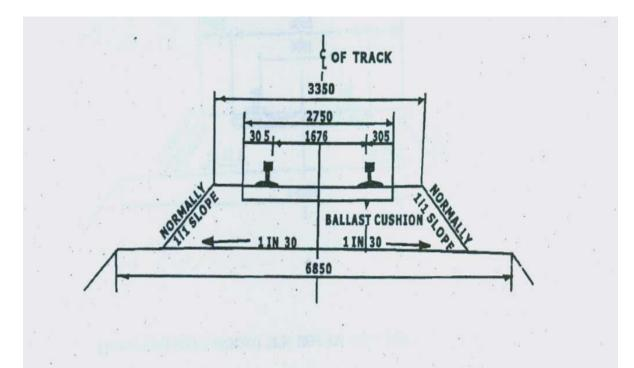
FIG. 4.1 STANDARD BALLAST PROFILE FOR BG SINGLE LINE TRACK (other than LWR / CWR)
